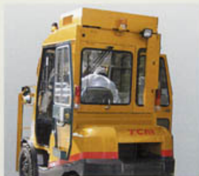
Steel cabin-enclosed type with air-cooler (available for 2-3.5ton models)
