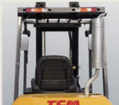
Overhead exhaust system
